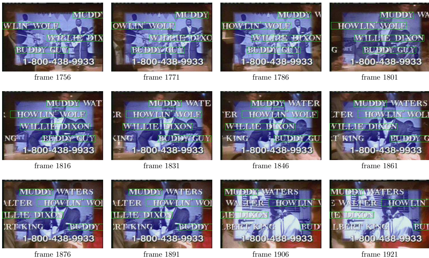
Fig. 3.4. Tracking algorithm applied to “scrolling7.mpg” video sequence with horizontally-scrolling text entering and exiting the frame.
