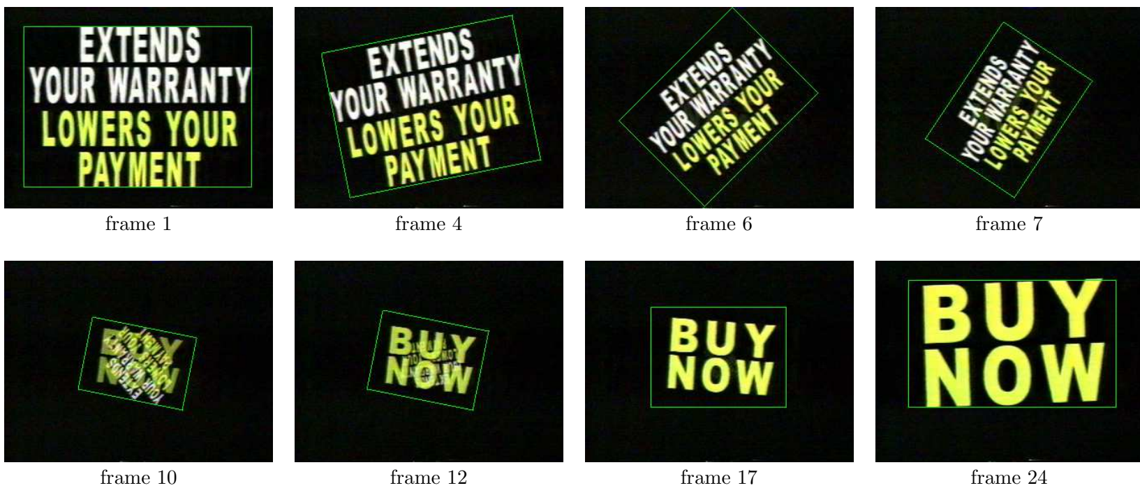
Fig. 3.11. Sample results of combined text detection and tracking on growing, shrinking, and rotating text.
