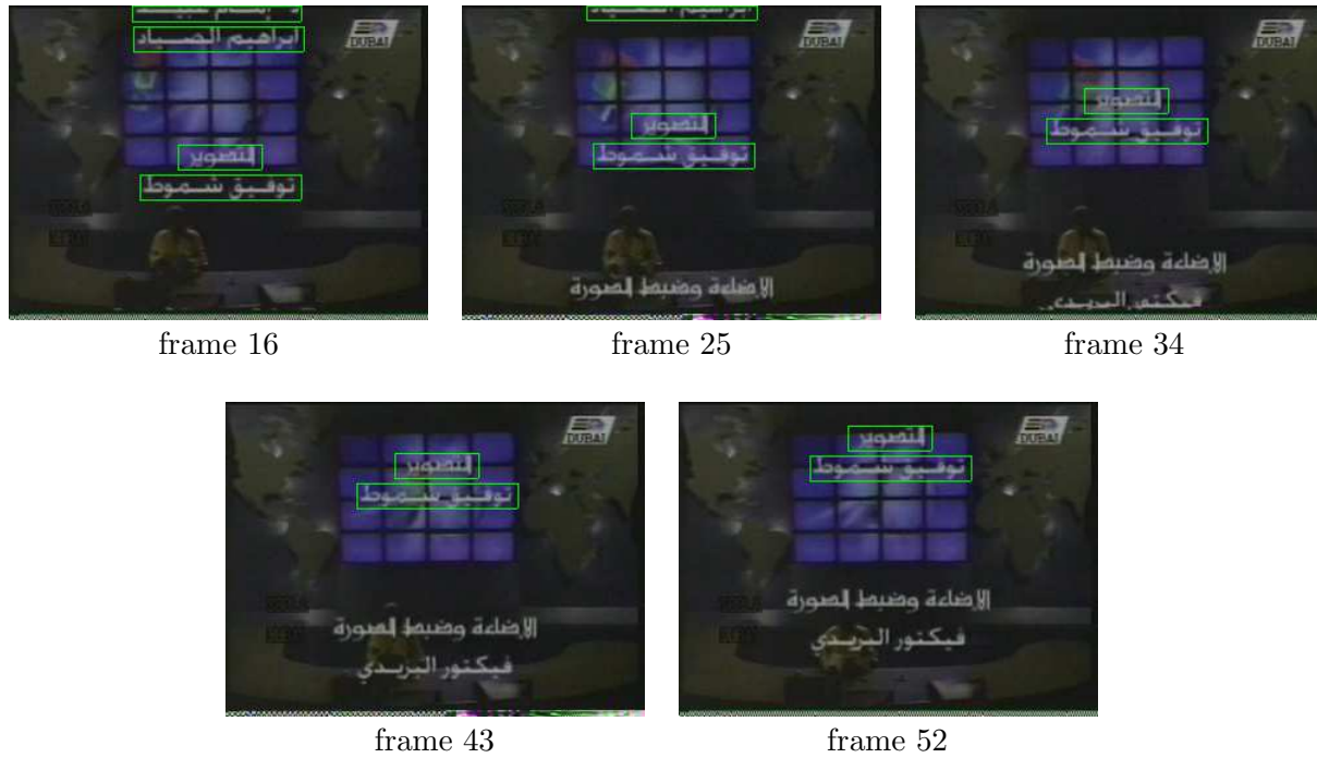
Fig. 3.5. Tracking algorithm applied to “t4.mpg” video sequence with vertically-scrolling caption text.
