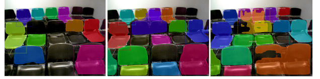
Fig. 5: Detection masks on three successive frames in a video sequence. Notice that the detector fires inconsistently on the same instance of “chair” object category. Our formulation can handle this noise with a unary term \phi(\cdot) that encourages temporal consistency across frames.
