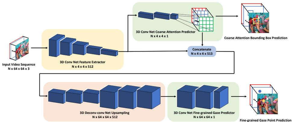
Figure 1: The architecture of our proposed two-stage 3D fully convolutional network model for eye gaze prediction. The number below each component indicates its output dimension, where  $N$  is the length of the input video sequence.
